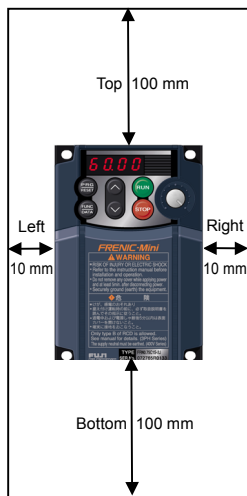
Figure 2.1 Mounting Direction and Required Clearances
