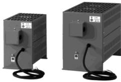
If the drive wire for the motor is long, an extremely low surge voltage (micro surge) occurs at the wire end connected to the motor. Surge voltage causes motor degradation, insulation breakdown, or increased noises. The surge suppression unit (SSU) suppresses the surge voltage. It features the connectivity for all inverter capacities and easy wiring work.
