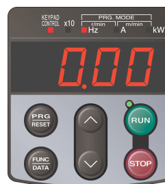
Figure 4.3 Display of the LED Monitor after Power-on
